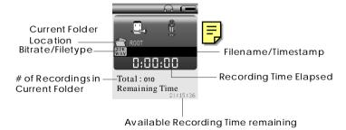
To change the recording quality (i.e., bitrate/filetype) options, press the JOYSTICK SELECT key while the recorder is stopped.
